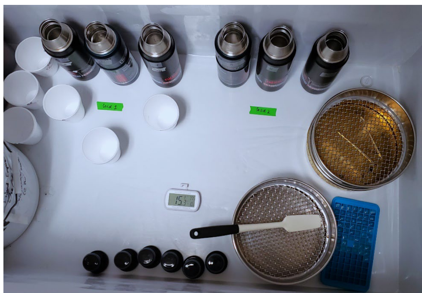
Figure 4. Freezer with thermoses and lids, Styrofoam cups, sieves with pans, brush, ice cube tray, and digital thermometer set up for testing.
