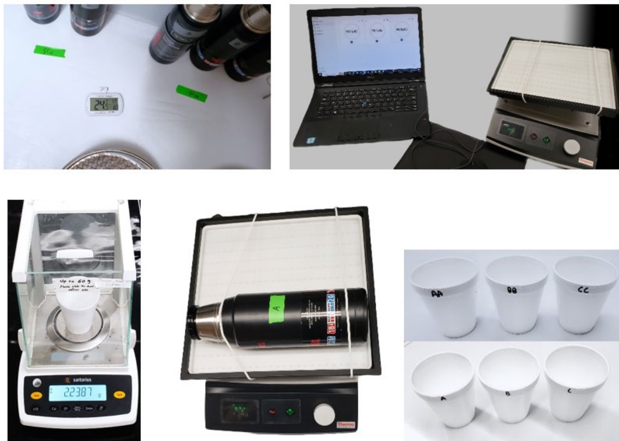
Figure 28. Modified IMCRT: a thermometer showing a test temperature (top left), laptop used for timers (top right), high accuracy weighing balance (bottom left), the Rocker and labeled thermos (bottom middle), and Styrofoam cups used and labeled (bottom right)
