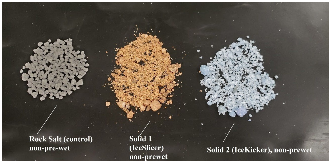
Figure 32. Solid salt samples: Solid control – rock salt (left), Solid 1 – Ice Slicer (middle), and Solid 2 – IceKicker (right); showing variation in gradation, particle size distribution.
