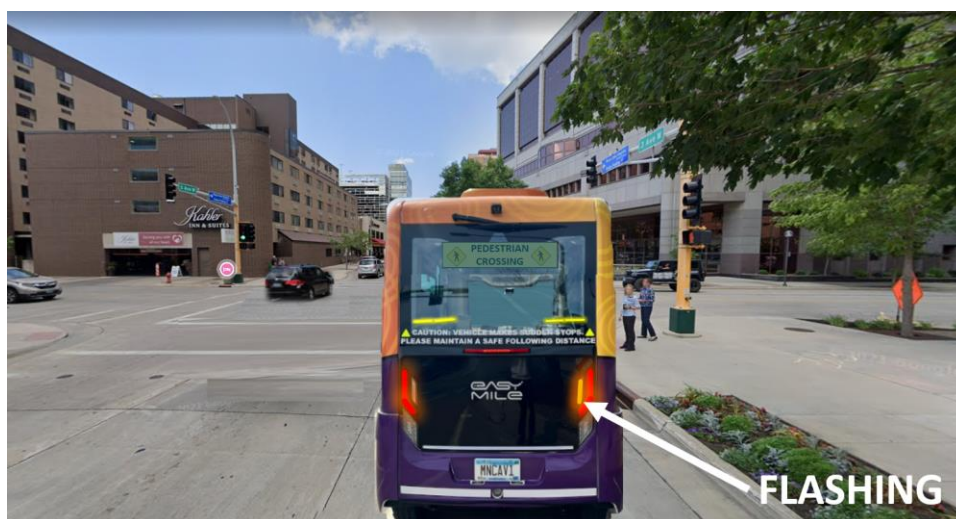
Figure 4.6 Turn signal and an LED screen displaying crossing icon and text “PEDESTRIAN CROSSING”
