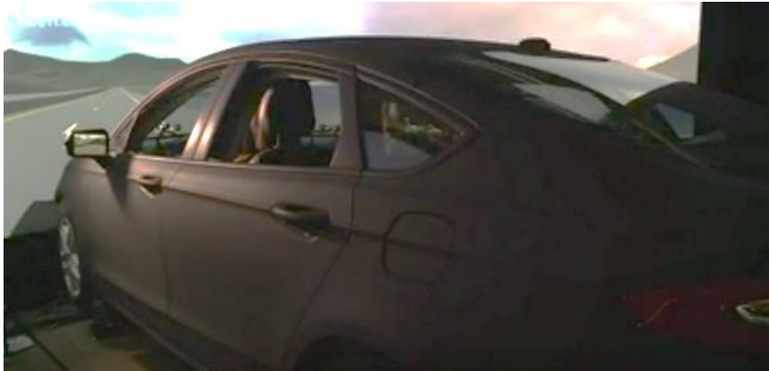
Figure 5.4 HumanFIRST immersive driving simulator
