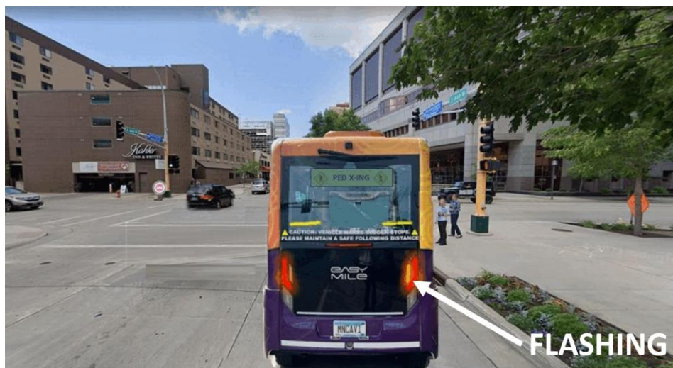
Figure 4.5 Turn signal and an LED screen displaying crossing icon and text “PED X-ING”
