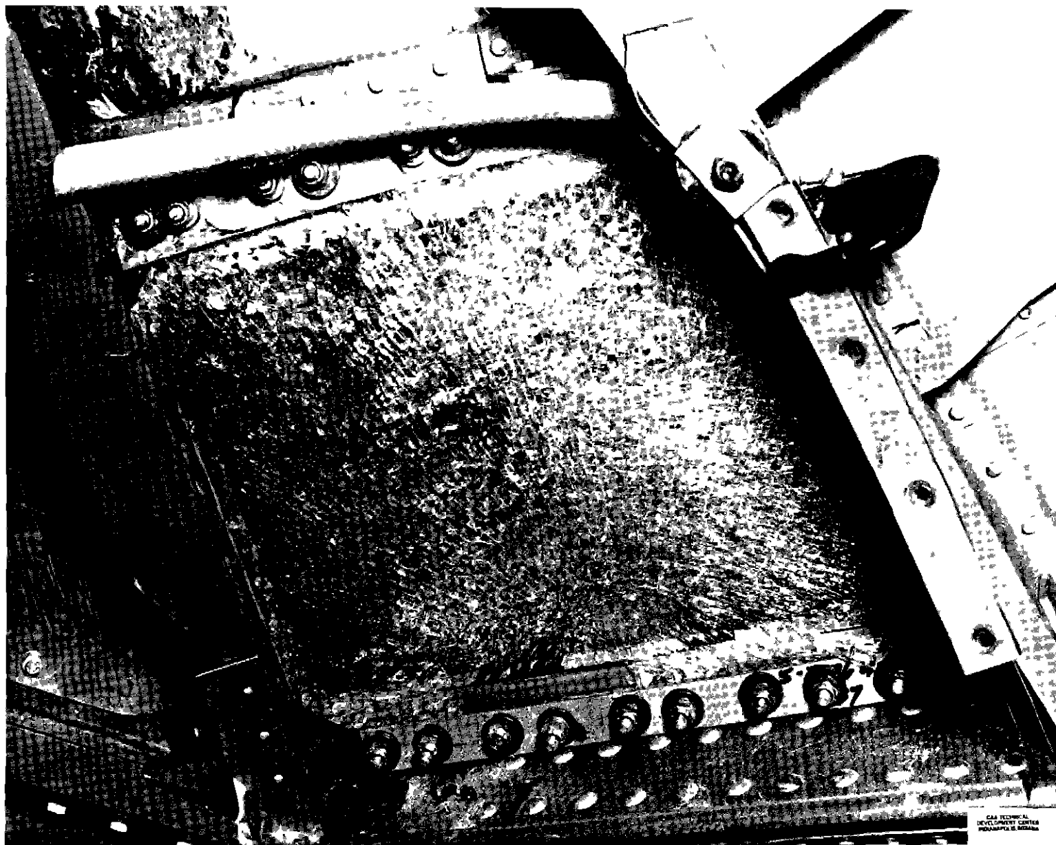
FIG. 36 - TEST NO. 14 - 7/22/56 - BIRD-CARCASS VELOCITY 405 mph
