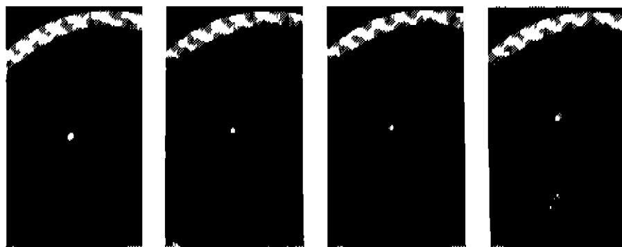
SUCCESSIVE SCANS OF 18-FOOT ANTENNA DISPLAY SHOWING TWO AIRCRAFT TARGETS IN HOLDING PATTERN. ONE TARGET FADES OUT DURING TURN THEN REAPPEARS IN LAST PICTURE
