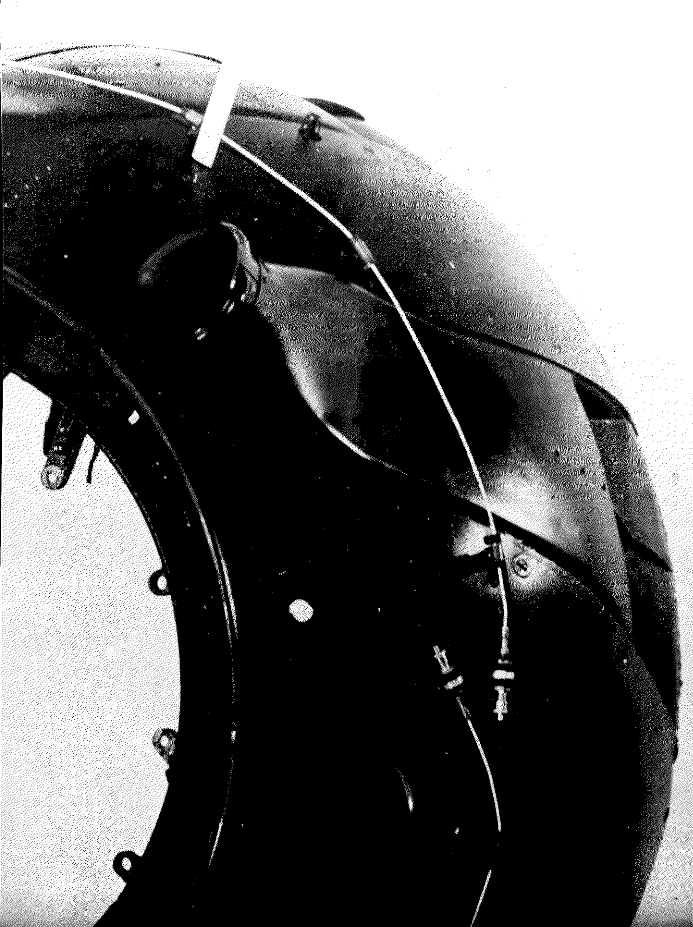
FIG. 8 MOUNTING DETAILS FOR AFTERBODY LOOP
