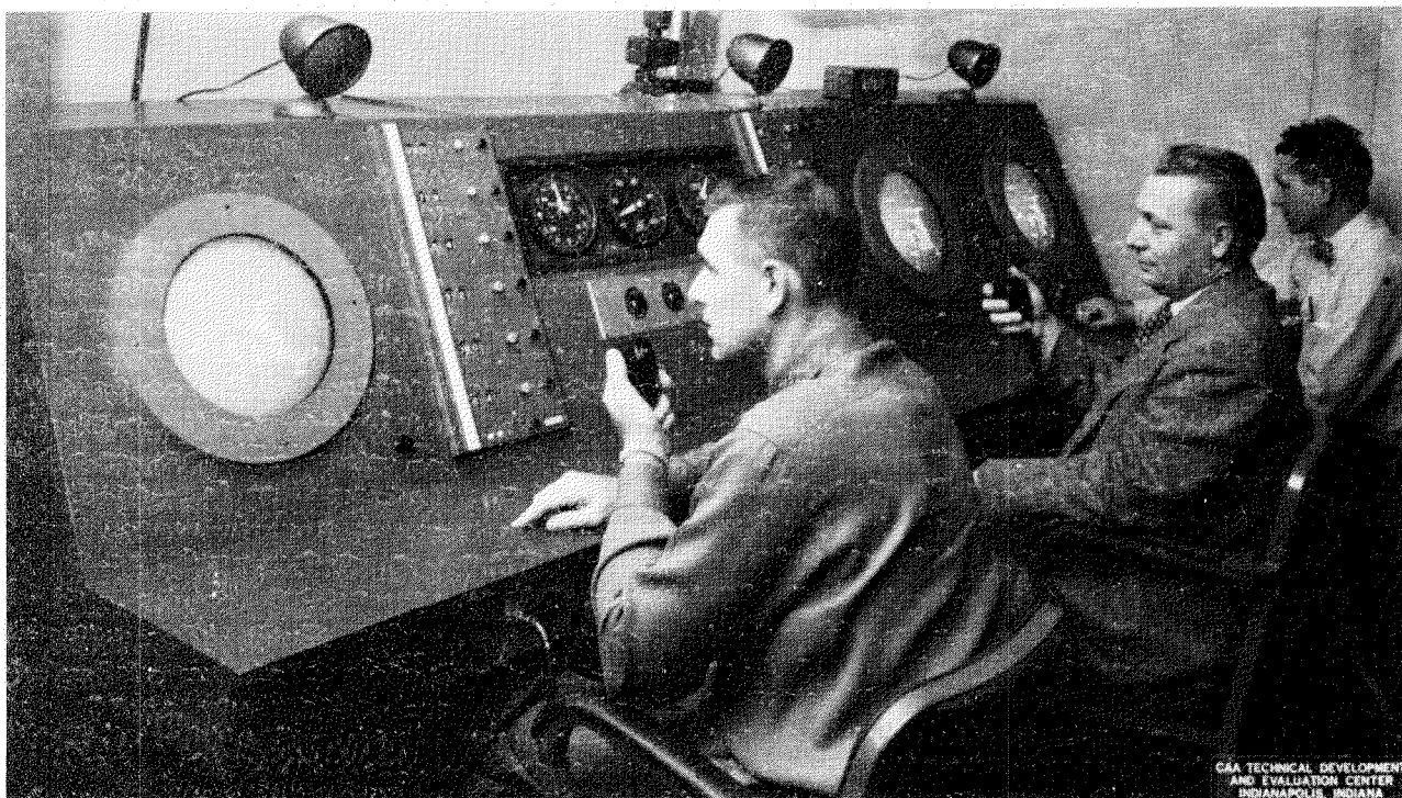
Fig. 1. Control Desks Showing the Simulated Radar Displays and the Data-Transfer Equipment
