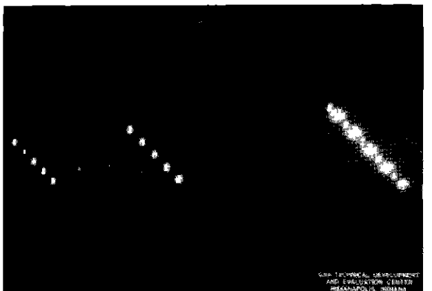
Fig 4C Slope Line Approach Lights Photographed Through Windshield Treated with Anti-Wetting Agent Rainfall 2.4 Inches Per Hour
