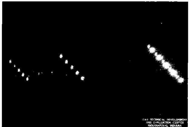
Fig 4B Slope Line Approach Lights Photographed Through Windshield Treated with Anti-Wetting Agent Rainfall 1.5 Inches Per Hour
