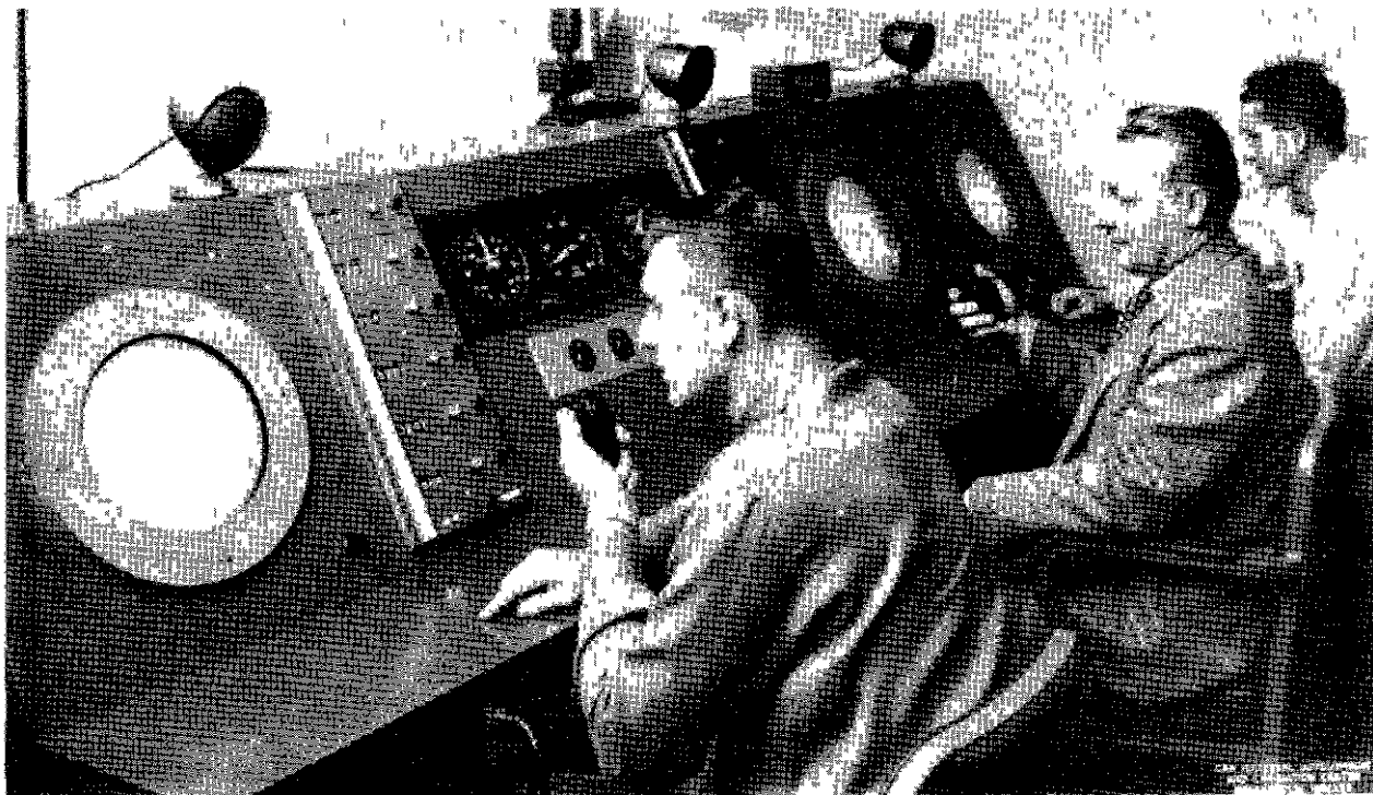
Fig 3 Dynamic-Simulator Control Desk With Simulated Radar Displays of Traffic Situation (For Norfolk evaluation tests the central portion of the desk between the radar scopes was replaced by a standard 5-board ARTC sector-control desk. Each of the three radar controllers was provided with a small flight-progress board.)
