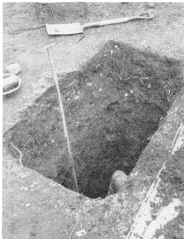
Fig. 13 The Excavation at Test Site. The Tube for Moisture and Density Measurements is Seen on One Wall
