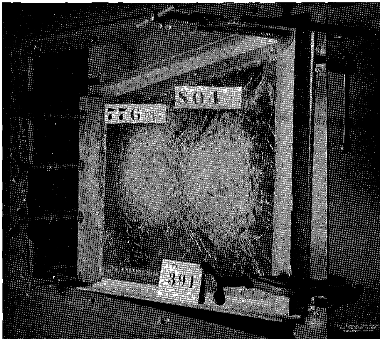
Fig 6 Results of Tests With 1 88-Inch Ice Spheres on a 0 188-Inch Vinyl Plastic Laminated Windshield Pane at 80°F and 60° Slope
