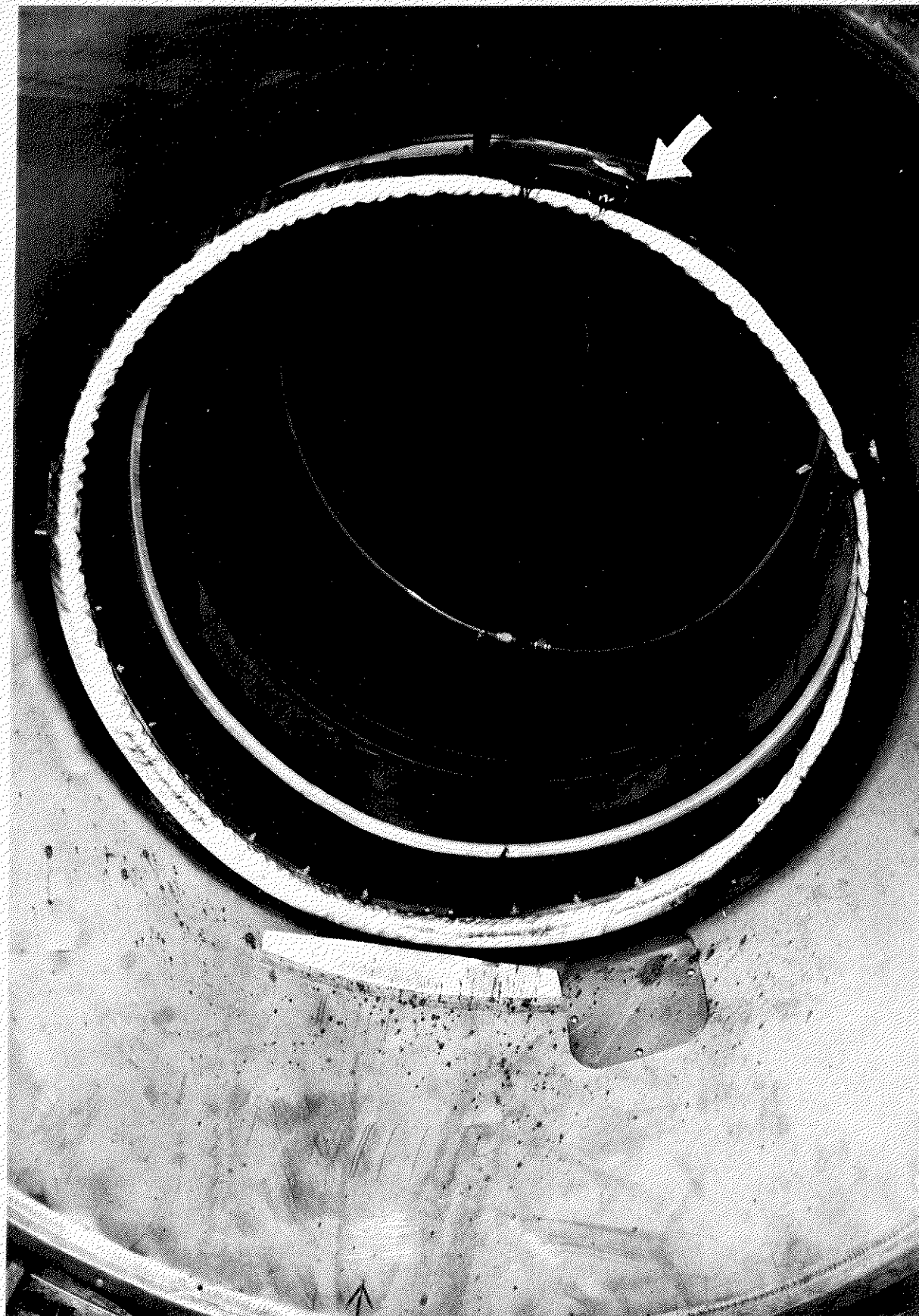
FIG.10 VIEW OF SCREEN SHOWING LOCATION OF FAILURE — RESTRICTED —
