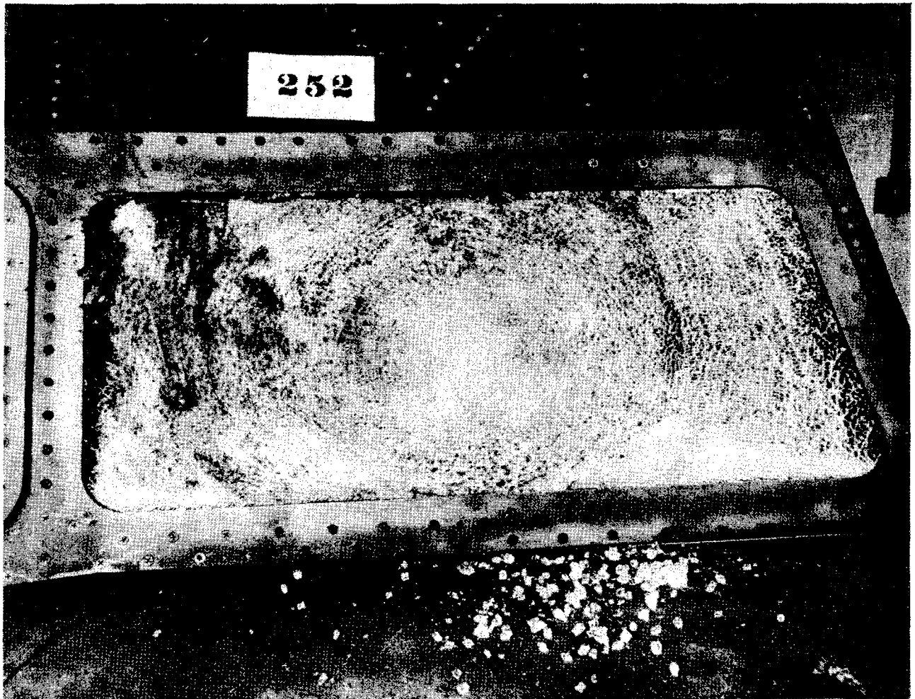
Fig. 12 Impact Test Resulting in Nonfailure of a Douglas DC-6 Windshield Utilizing 3/16-in. Polyvinyl Butyral Interlayer Tested With 4-lb. Chicken Carcass at 300 mph
