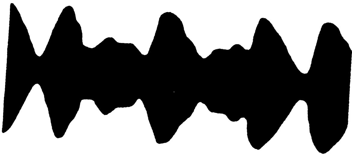
FIGURE 97. Sketch of Oscillograph Pattern for Localizer on-Course Signal.
