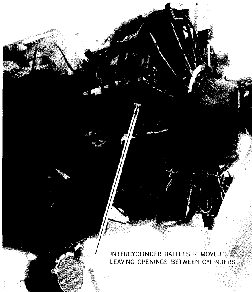
FIGURE 5. Powerplant installation (right side) after 1200 fires. Arrow shows opening between cylinders due to the removal of the intercyylinder baffles as described under "General Test Procedure".
