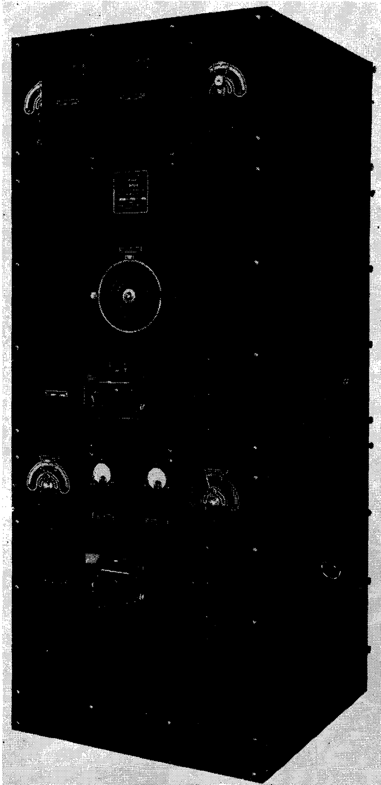
Figure 12.—Front View of Radio Range Coupling Unit.
