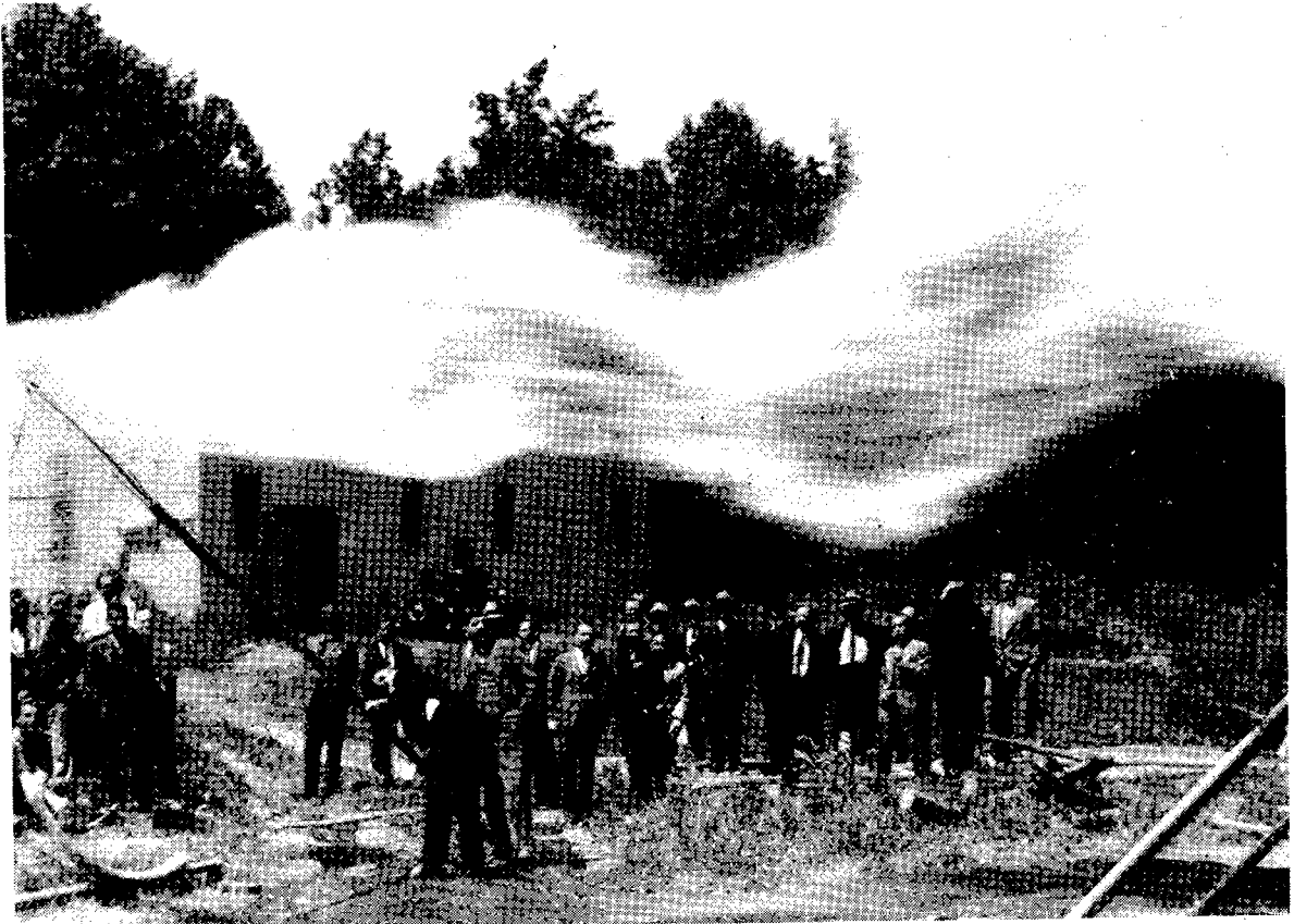
Figure 5.—Gasoline spray burning in free airstream with ignitor in place.
