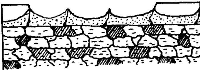
Fig. 2 Schematic cross section showing corrosion attack extending to the diffusion zone.
