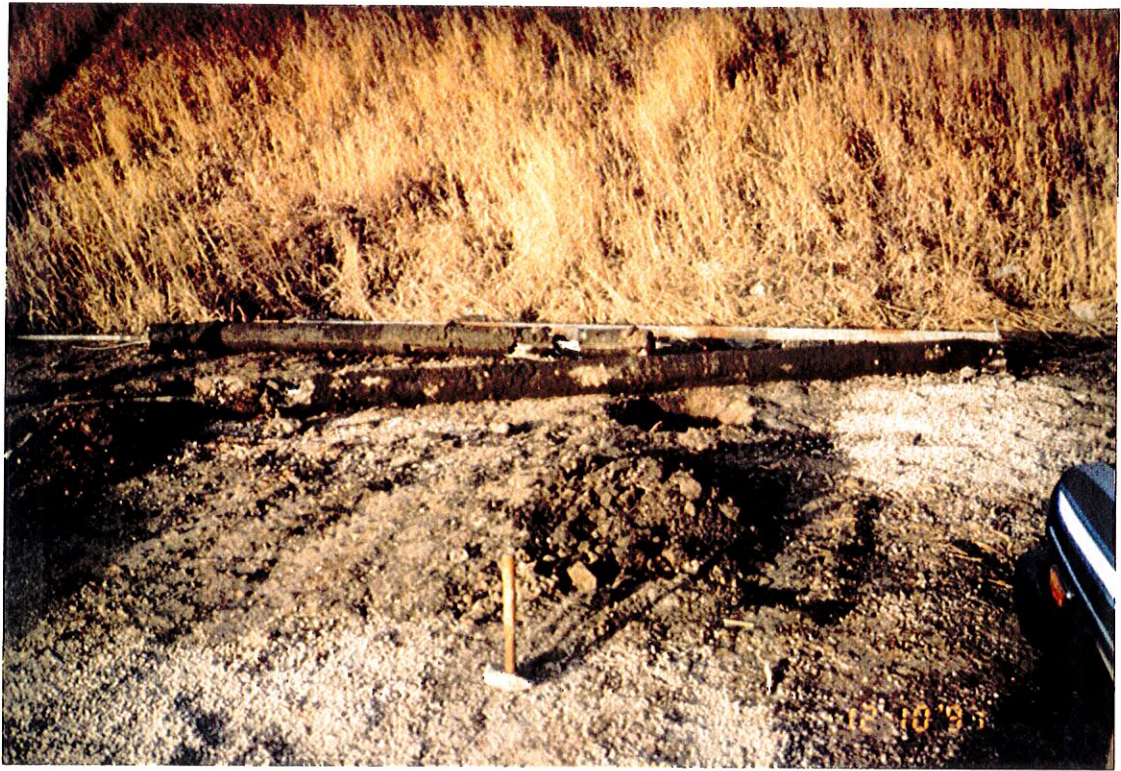
Figure 4-8. Excavated Test Shafts with Voids, Site A.
