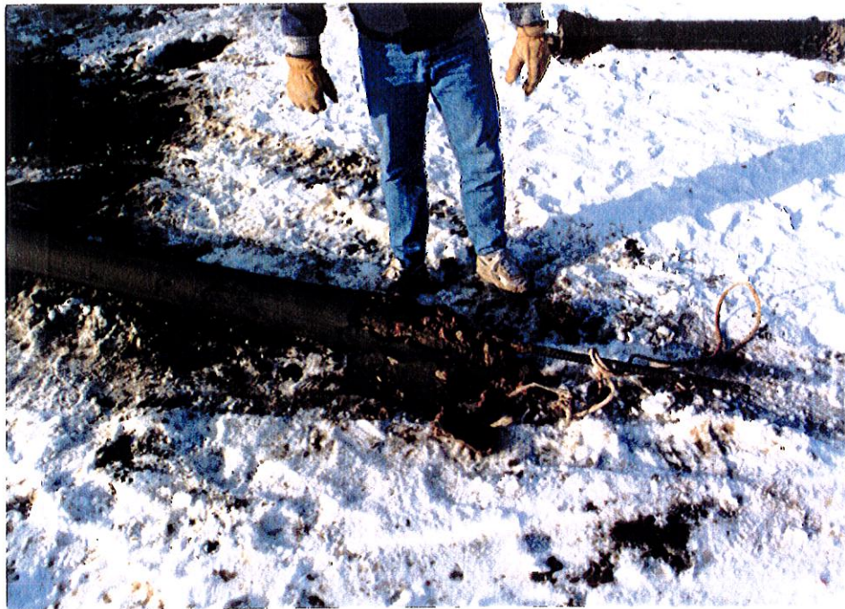
Figure 4-9. Test Shaft A2 Following Excavation Showing 2.2. ft. Void at Tip.
