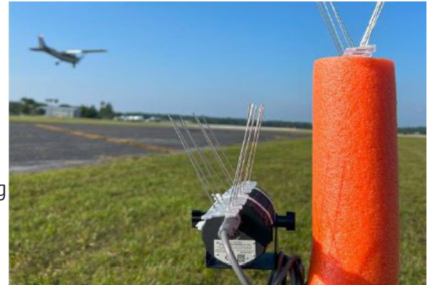
Sensors like this one may capture non-cooperative targets like take-off and landing operations using position and speed measurements.
