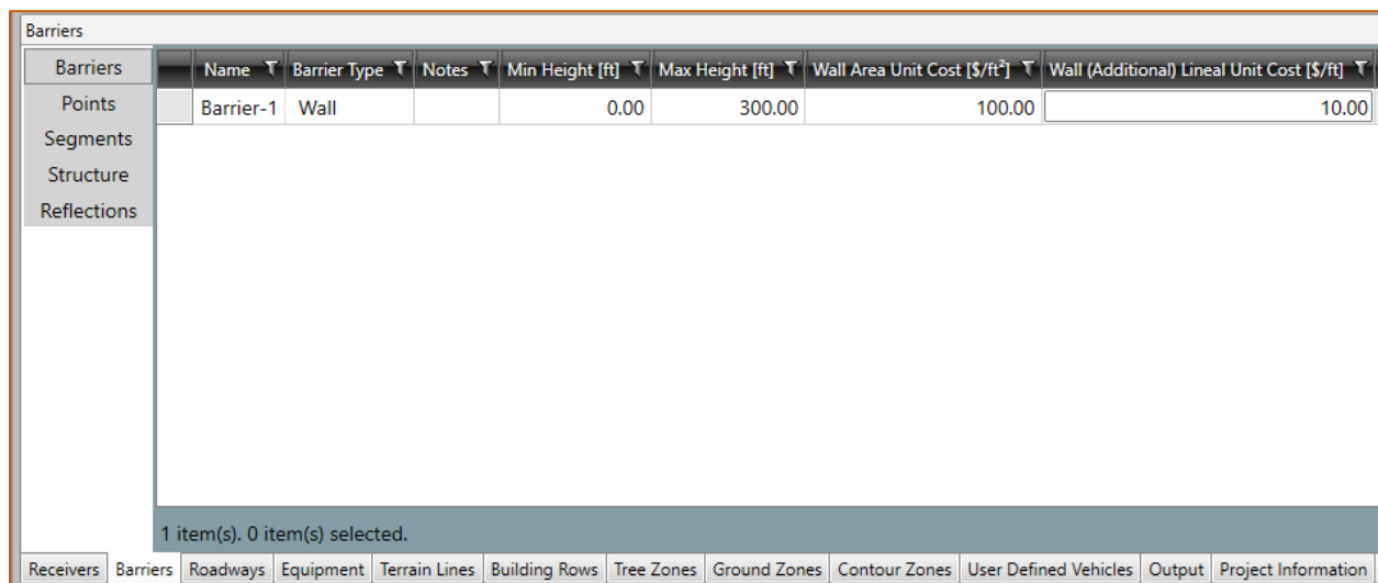
Figure 33 Barriers tab in the Object Details Pane with appropriate barrier costs
