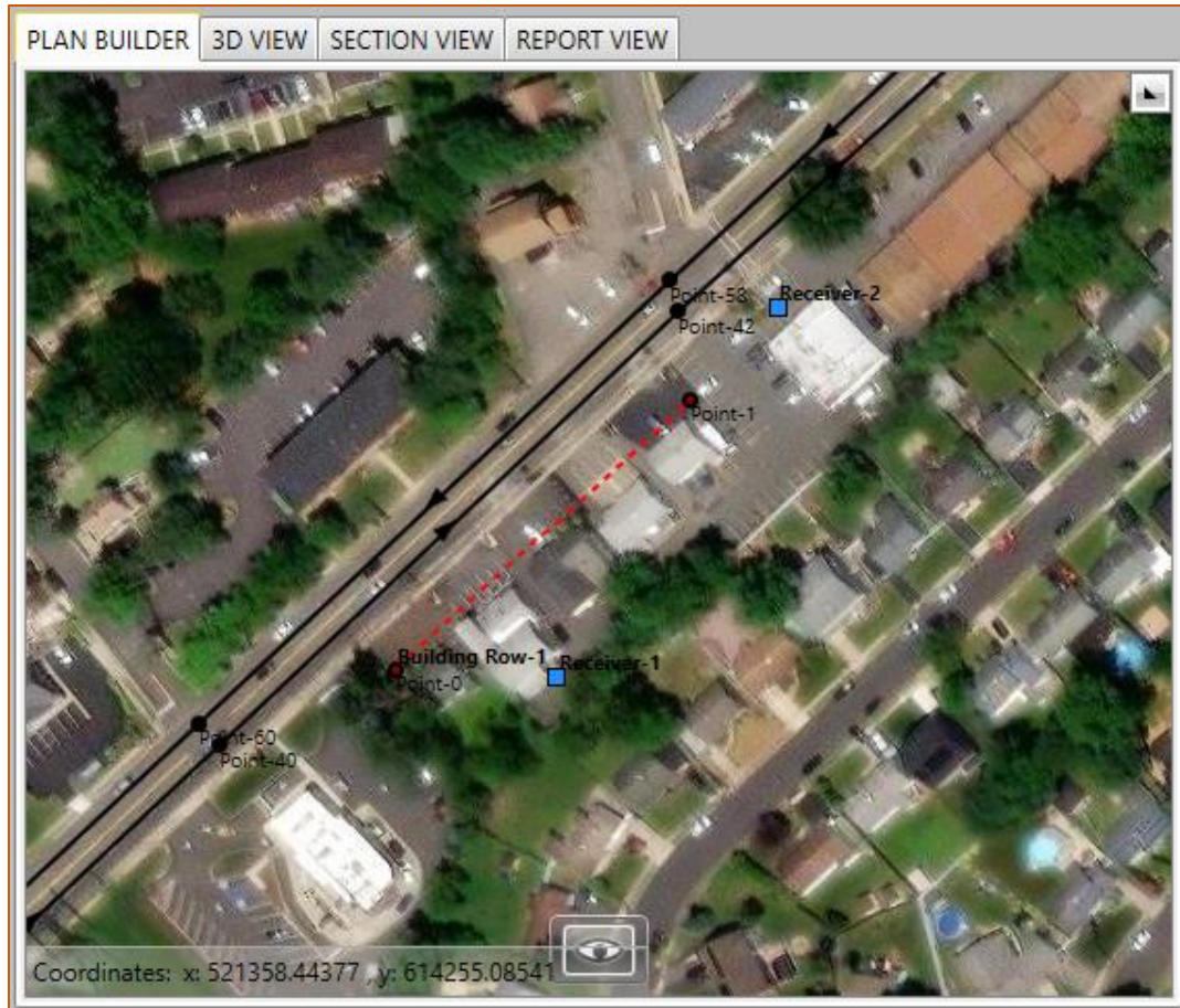
Figure 19 Plan Builder with two roadways, two receivers, and a building row on the Aerial View basemap
