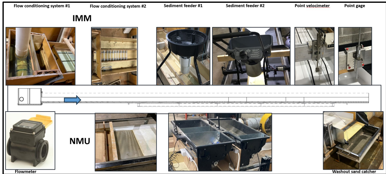
Figure 19. Essential items for flow control and experiment execution for the IMM and NMU tests
