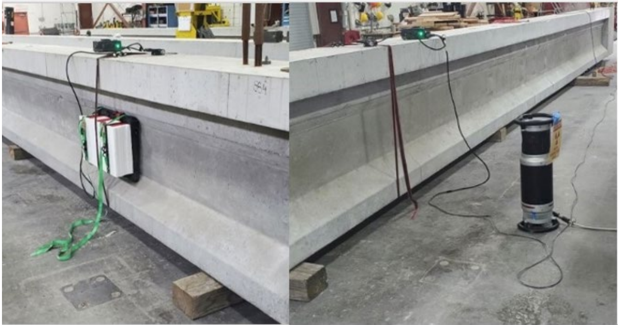
Figure 90. YXLON X-Ray machine on internal duct specimen
