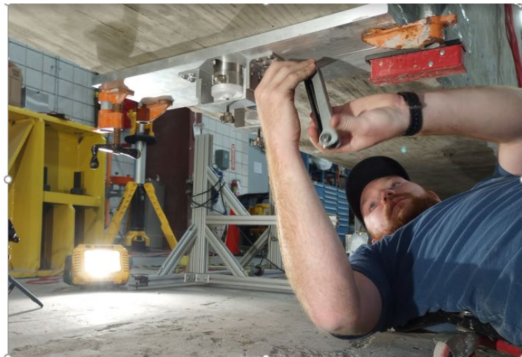
Figure 134. Fixture for mounting transducers using two-part epoxy
