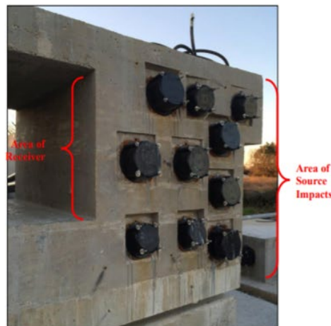
Figure 43. Testing area for UPV and SPV testing performed by Hurlebaus (Hurlebaus et al. 15 ).
