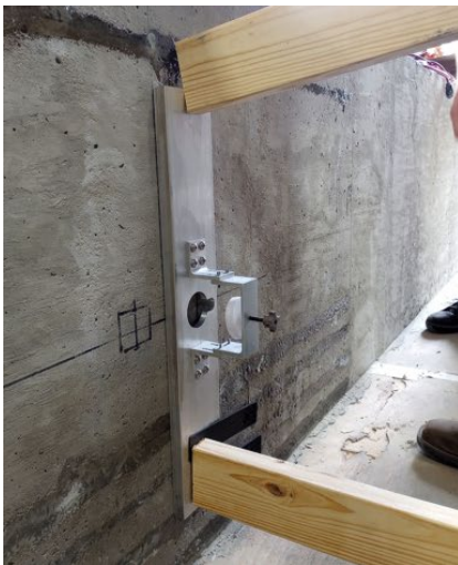
Figure 134. Fixture for mounting transducers using two-part epoxy
