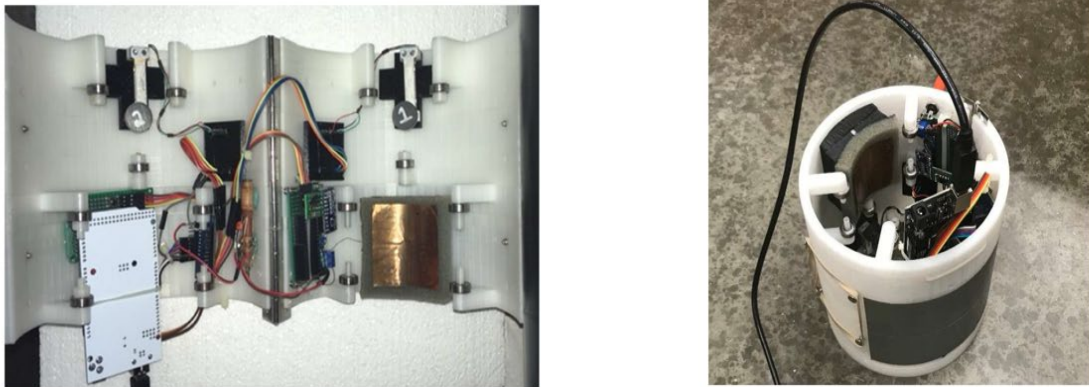
Figure 25. Layout of electronics for tendon imaging unit 10
