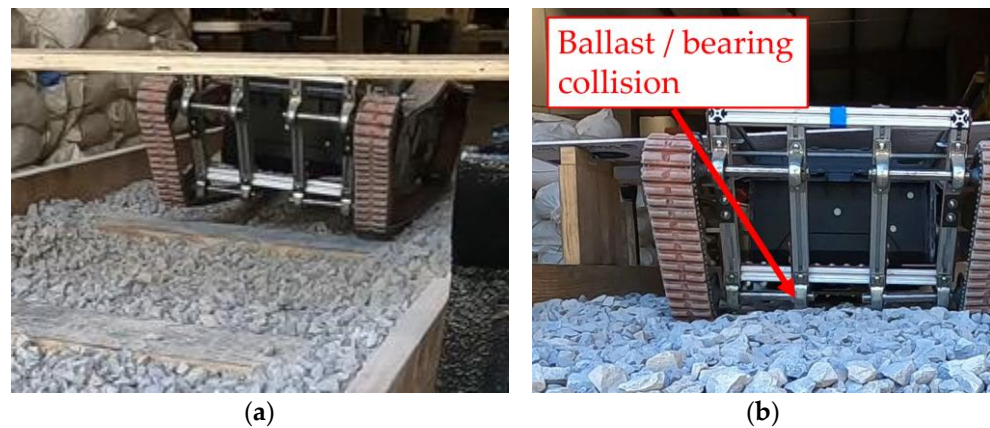
Figure 9. Test Bed evaluation results: (a) Sharp collision during the 6.8 km/h test, causing the front end of the TCR to become airborne; (b) Impact between the ballast and bearing housing.
