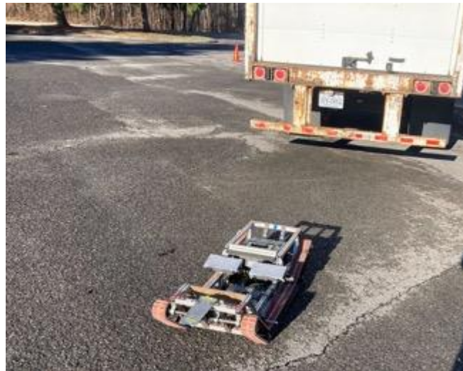
Figure 24. The setup for under-trailer testing. The light bars were relocated to the front transverse frame member and oriented vertically.
