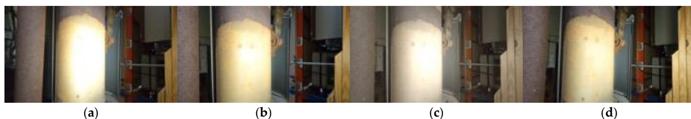
Figure 26. Comparison of diffusion methods on glare reduction from mufflers: (a) No diffusers; (b) Wax paper; (c) Plexiglass only*; (d) Plexiglass and wax paper. * Different color settings were used in other tests.
