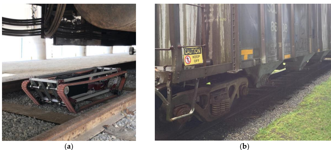
Figure 2. (a) The TCR operating on the track bed beneath a railcar; (b) A hopper railcar illustrating the low height of the gates above the track bed.
