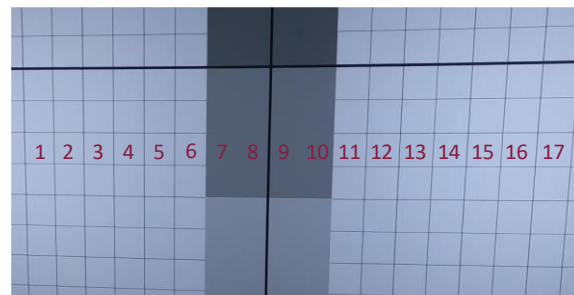
Figure 7. Existing field of view (FOV) evaluation image demonstrating an ability to image only 17 grids (430 mm) at the minimum height.
