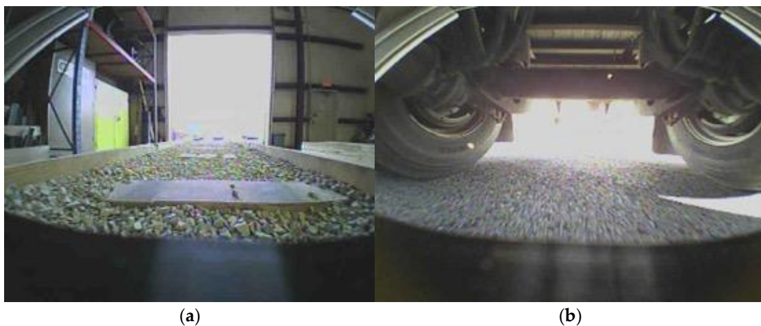
Figure 32. FPV testing results: (a) 4.8 km/h test over Test Bed showing the ability to operate in high vibratory conditions; (b) 9.6 km/h under the trailer showing a dark to light transition.
