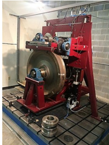
Figure 2-4 Isometric view of solid model (left), and fully assembled (right) VT – FRA Roller Rig
