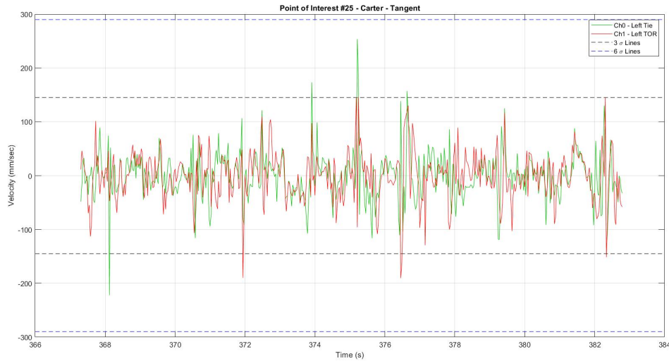
Figure 30: Carter Tangent High-pass filtered Doppler LIDAR Overview
