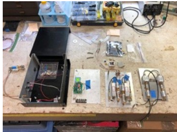
Figure 38: 2020 LIDAR RF unit under construction
