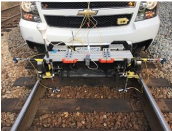
Figure 45: LIDAR Rig installed on NS Hy-rail truck with a mechanical gage sensor
