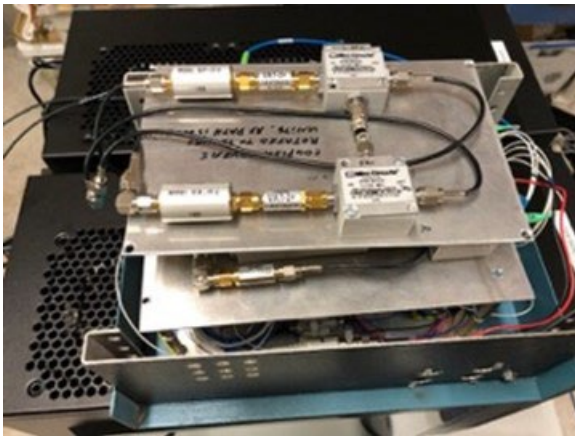
Figure 37: 2011 Integrated LIDAR RF unit
