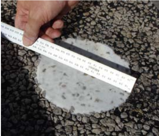
Figure 9. Measuring Four Diameters of the Resulting Circle for Averaging.
