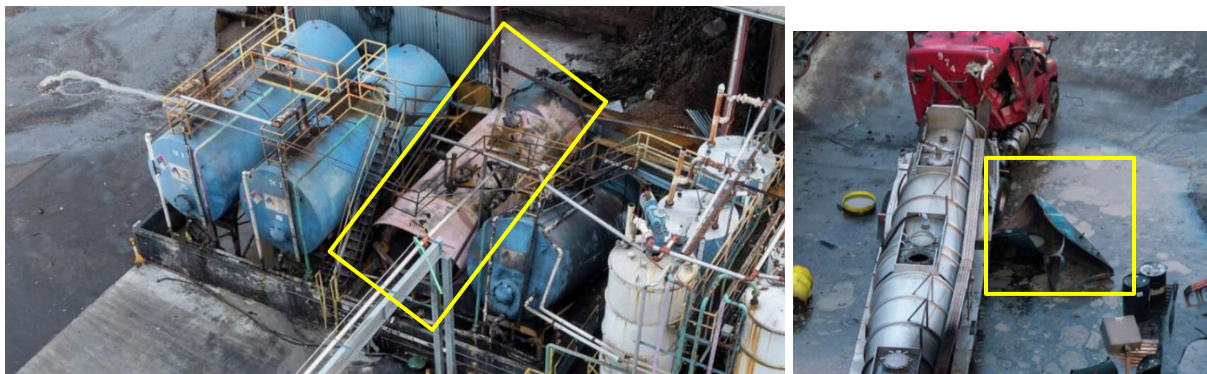
Figure 1. The tank that exploded (left). A portion of the tank after the explosion (right) (Credit: Tradebe, annotated by the CSB).
