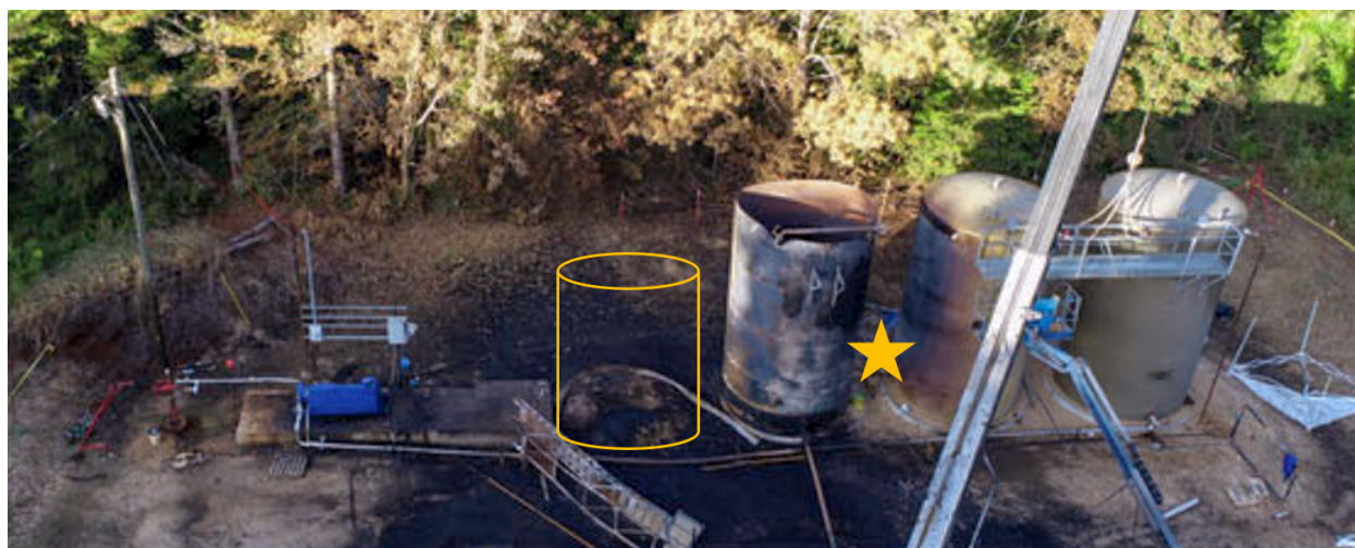
Figure 3. This post-incident photo shows the location of the welding activity that triggered the explosion (gold star) and the pre-incident location of the fourth tank, which was launched by the blast and propelled into the woods shown in the background. (Credit: Red Hancock with annotations by CSB)
