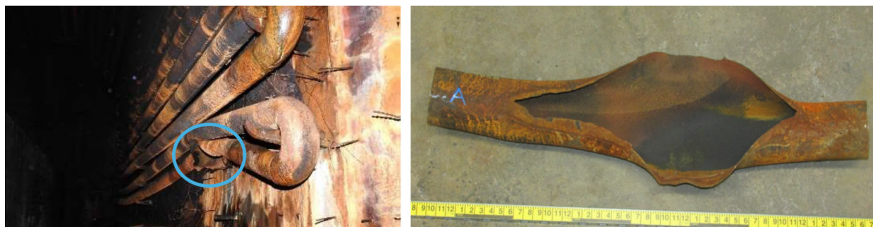
Figure 9. The ruptured tube within the fired heater (left) and after removal (right). (Credit: Delek)
