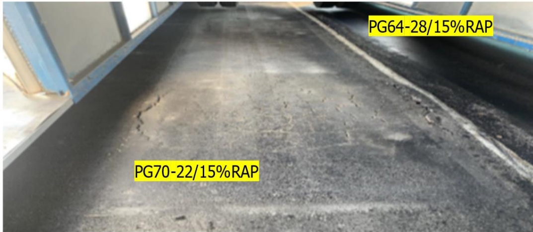
Figure 59. Fatigue Cracking on Test Section O with PG70-22 (Left) and Section P with PG64-28 (Right).
