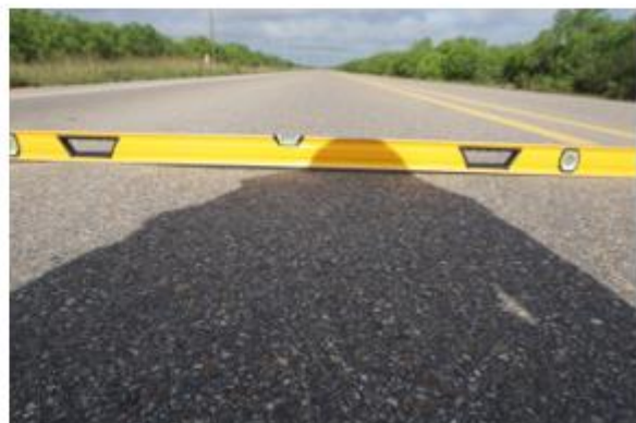
Rutting in Inner Wheel Path: 1/16–8/16 in. 03/29/2018
