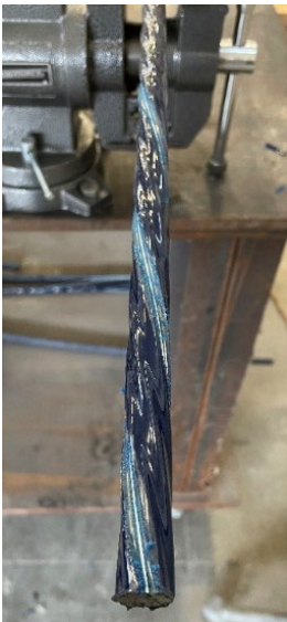
(c) Epoxy coating removed
