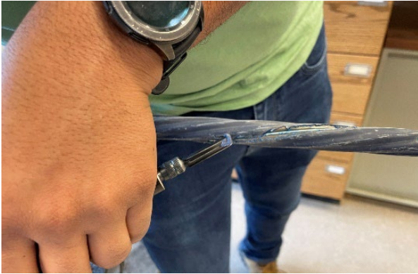
(b) Removing epoxy with electric chisel
