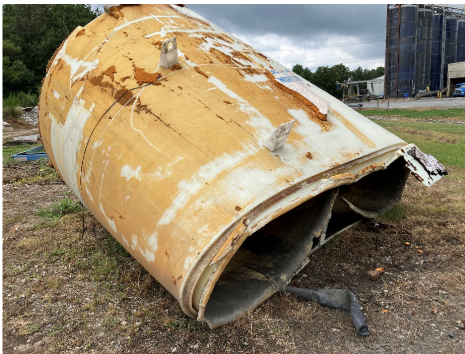
Figure 1. Ruptured Polyethylene Tank at Darling. (Credit: Darling)
