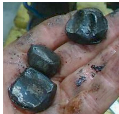
Figure 1. Damaged Pump Bearings. (Credit: Pemex)
