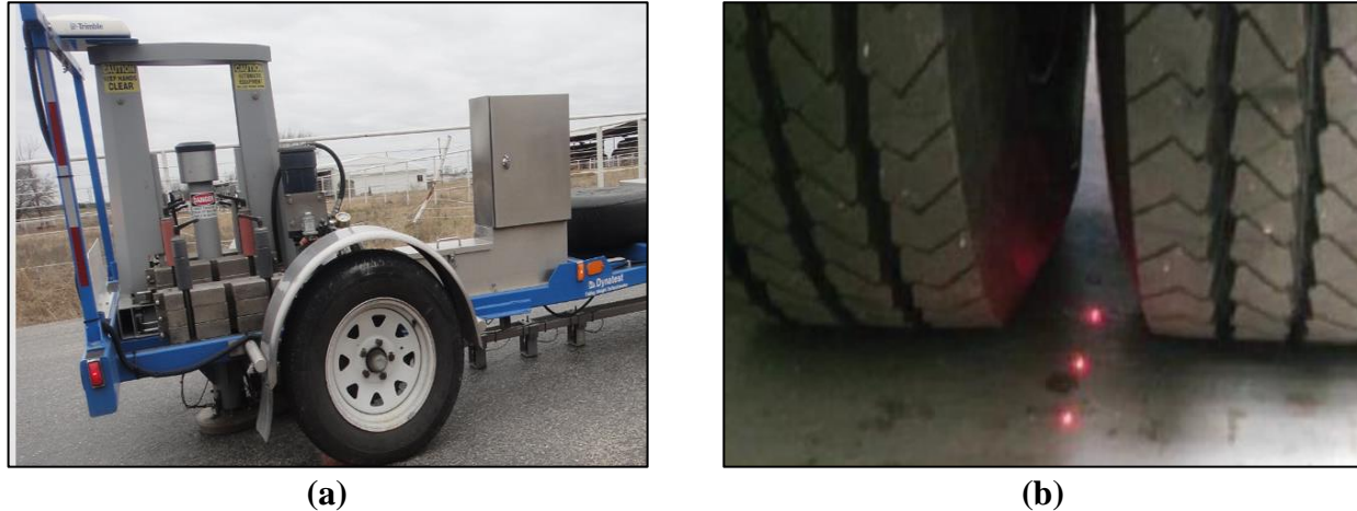
Figure 3. Device Operation Modes: (a) FWD Geophone and (b) TSD Laser Sensor Array [3].
