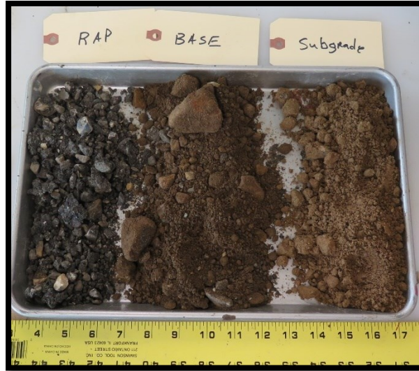
Figure 9. ATL US 80: (a) roadway sampling location, (b) representative materials.
