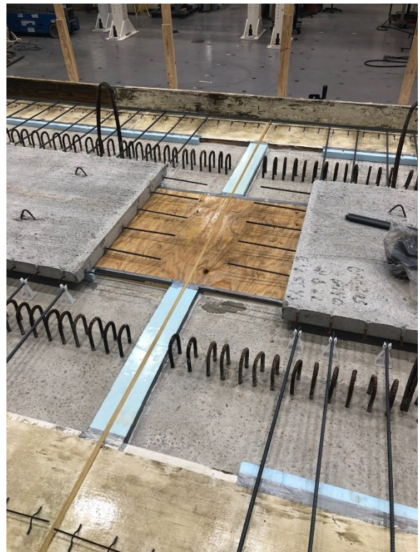
(b) With post-installed PCP dowels
