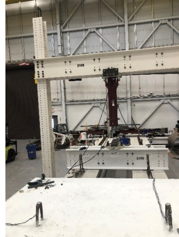
(b) East loading frame with spreader beam
