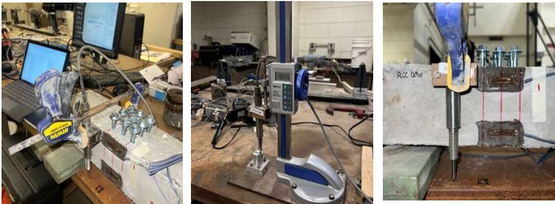
Figure 15: Deployable a 3 rows of 9-0.375 in. anchors being installed into the concrete specimen 4 [left]. LVDT displacement/voltage data collecting [center] and front view of the anchor installation with and LVDT sensor on specimen 4 [right].
