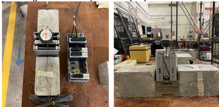
Figure 9: Experimental setup with the lab jack as the actuator.
