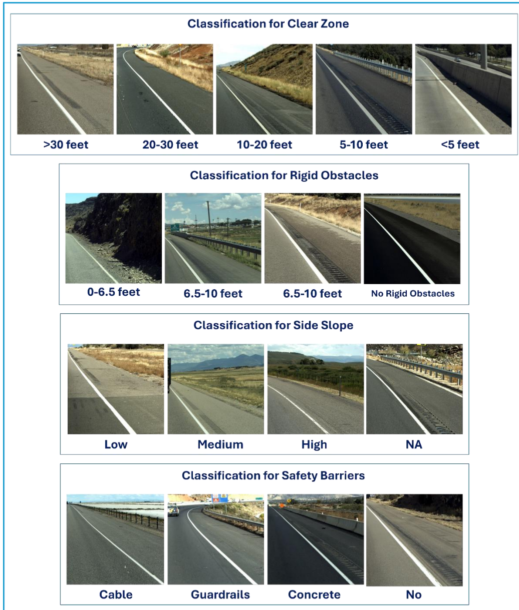
Figure 3.2: Categories and Examples for Labeling of Roadside Features
