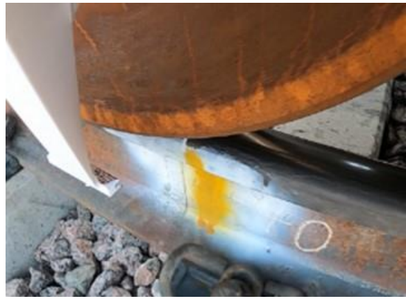
Welding defect 2: 0.3 in x 0.3 in. Location: 0.6 inches below the surface
