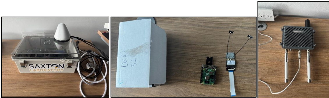
Figure 3. Photos. (left) DSRC OBU, (middle) the OwlBox open-source project used as U-NII-4 interferer, (right) DSRC RSU.
