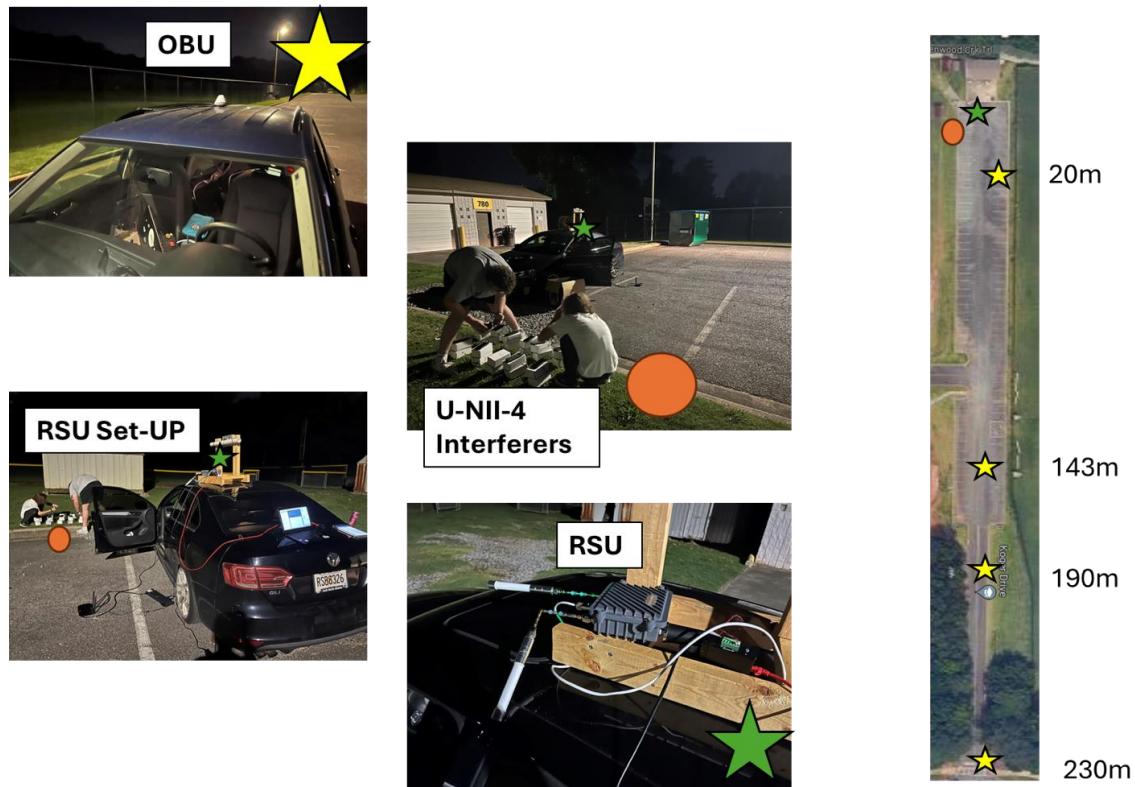
Figure 10. Photos. On campus field tests with a 20dB attenuator and 25 interferers to observe V2I and I2V range.
