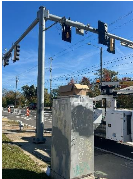
Figure 16. Photo. The U-NII-4 interferers closer to the RSU for the 2nd round of field tests conducted on 11/4/2024.
