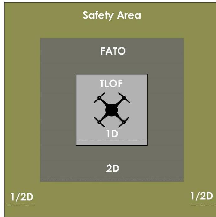
Figure 7.2 Relationship and Dimensions of TLOF, FATO, and Safety Area, Based on FAA Guidelines
