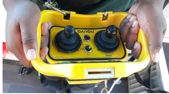
Attendant onboard the Navya Autonom operated by Beep in Cary's Bond Park (left); industrial controller used by the attendant onboard the Navya Autonom operated by Beep in Cary's Bond Park and at UNC Charlotte (right). (Images courtesy of NCDOT)
