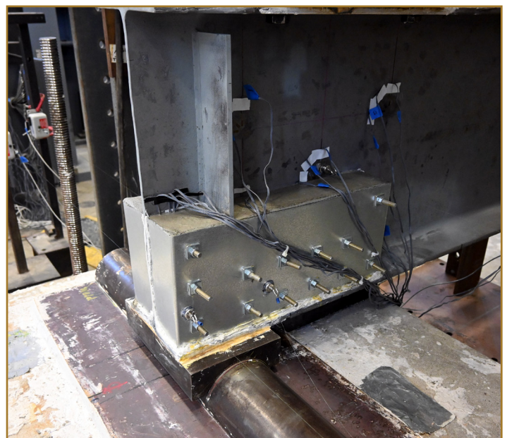
Repaired specimen using "Sandwich Panel" repair method.
