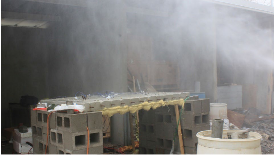
Figure 2.3 Creation of freezing mist via a snow gun
