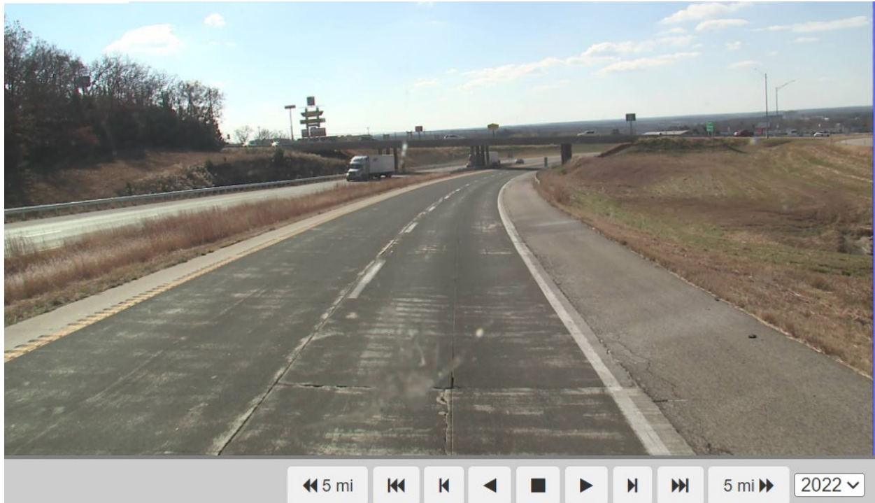
Figure 3-4: ARAN image of section 10 after HFST application (source: MoDOT)
