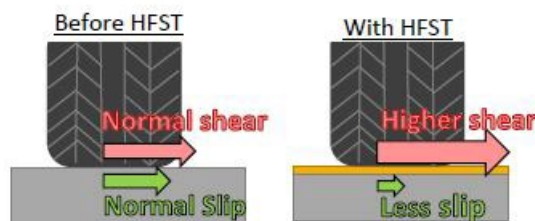
(c) Shear and slipping illustration
