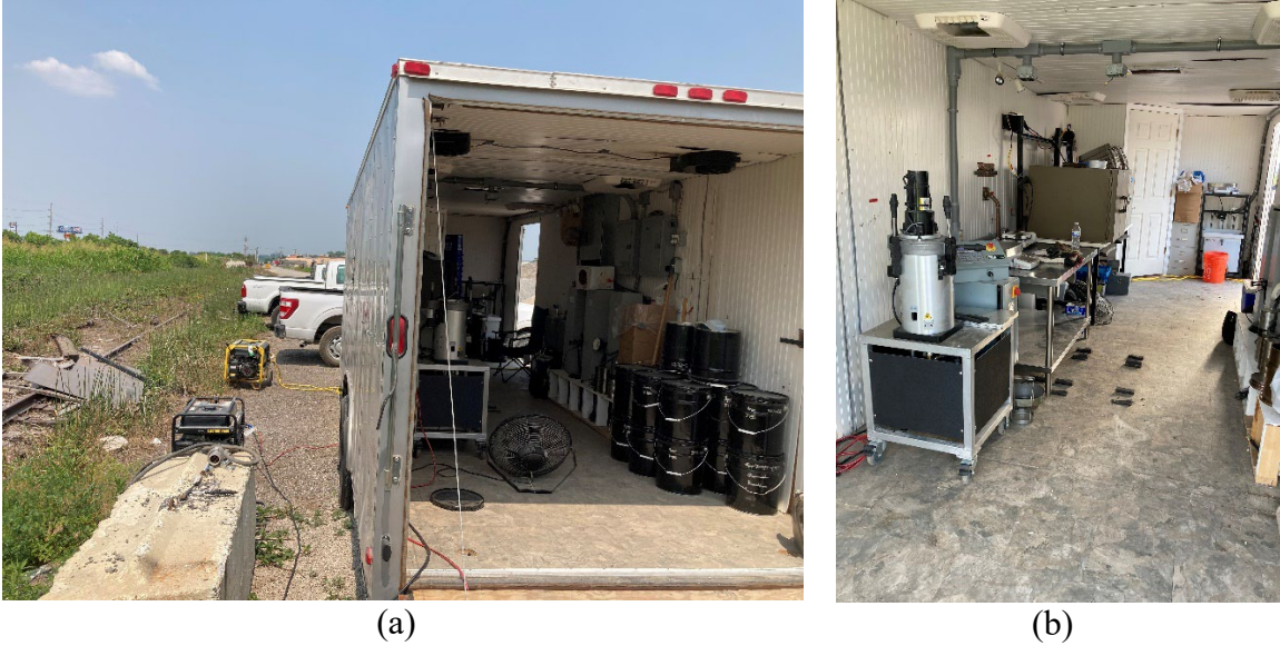
Figure 5.1. (a) MAPIL's mobile asphalt testing laboratory, (b) Machine setup inside the mobile laboratory
