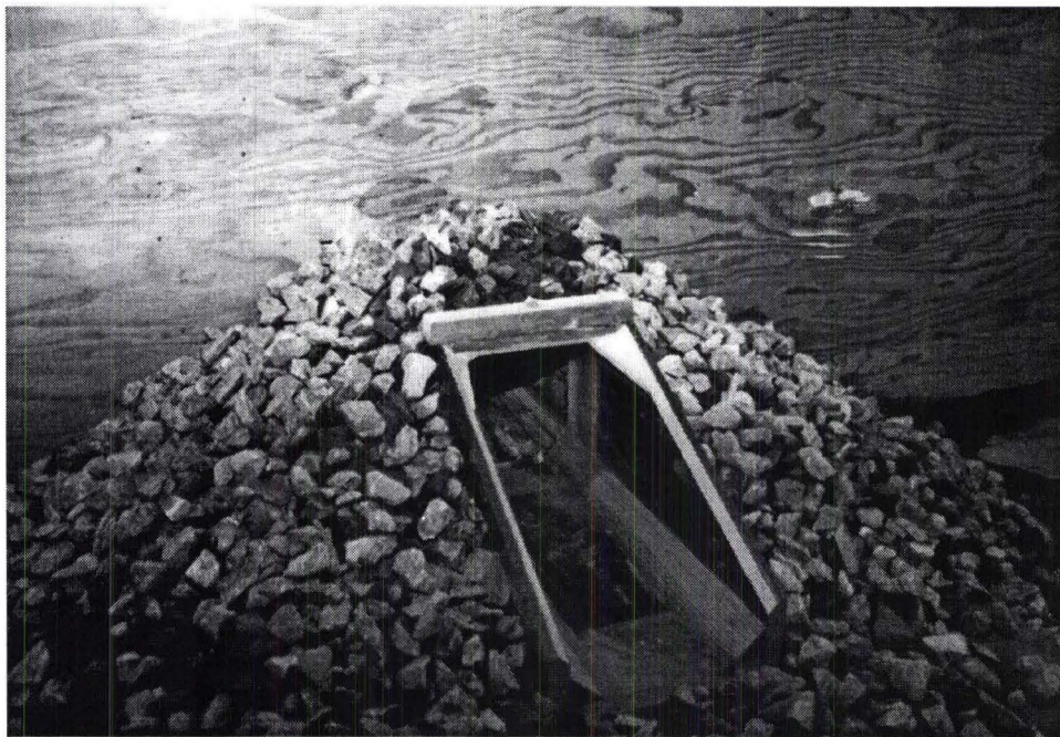
Figure 9. Culvert model 5, 6 ft x 6 ft precast, 0-degree wingwall flare.
