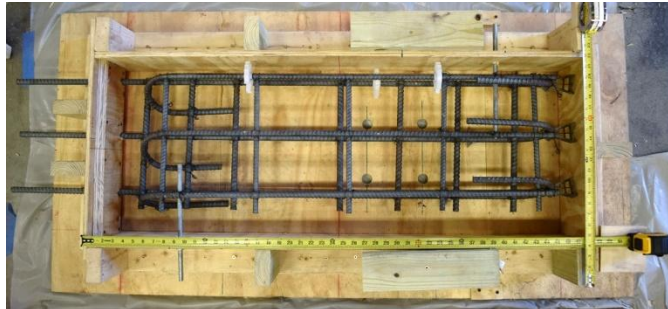
(a) NC formwork for slab specimens
