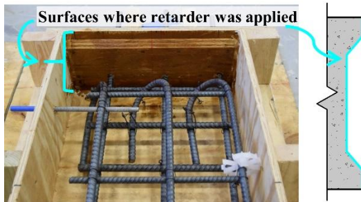
(c) Joint surface in NC formwork for slab specimens
