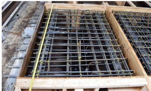
(e) NC formwork for double-tee specimens
