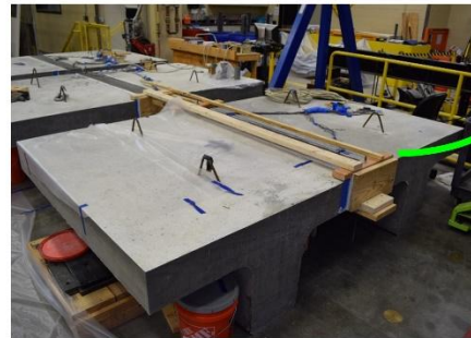
(e) Double-tee specimen with UHPC joint formwork
