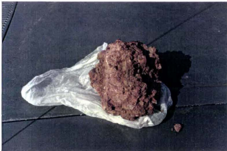
Photo V-35. Rapid City, Second Street - Degraded and Cemented Limestone Ballast.
