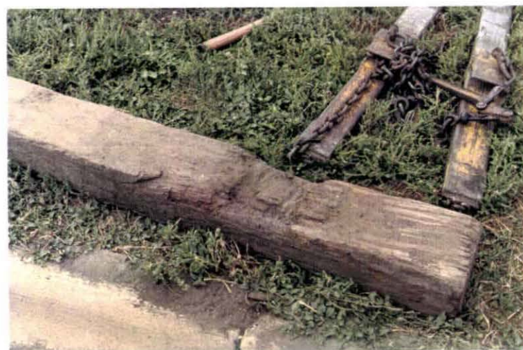
Photo V-20. Aberdeen, 12 Street - Deteriorated Tie.
