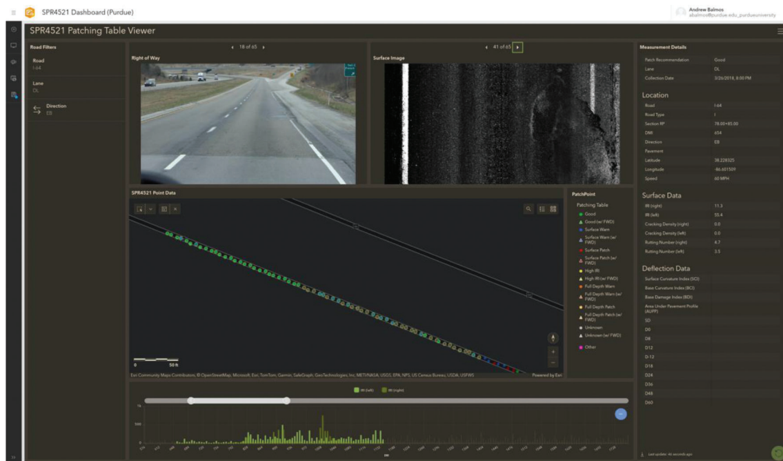
Figure 7.7 By selecting a small number of locations of interest, one can “click through” the set of ROW and surface images to explain and/or validate patching recommendations. In this case, the sudden spike of IRI can be accounted for by noticing that the road transitions from new to old, formerly patched pavement.
