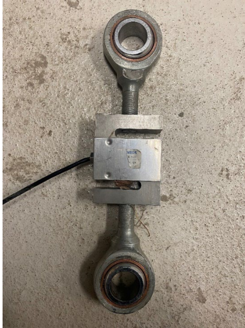
Figure 4.3 Tension S beam load cell with a capacity of 10 kips used in the static tests
