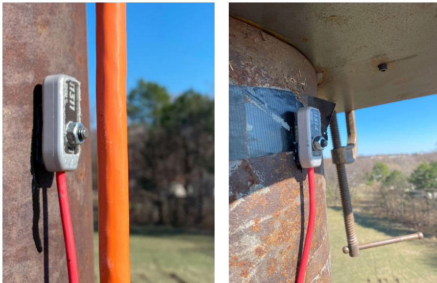
Figure 4.18 The installation of BDI accelerometers on the poles to measure the acceleration during forced vibration test
