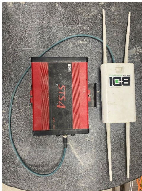
Figure 4.6 STS4 Wireless Base Station
