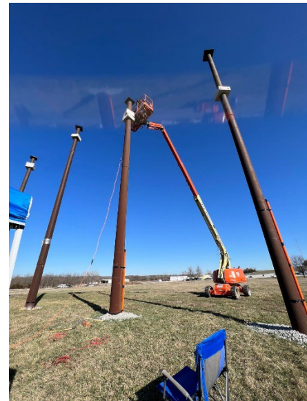
Figure 4.16 Installation of the shaker at the top of each pole before the forced vibration test
