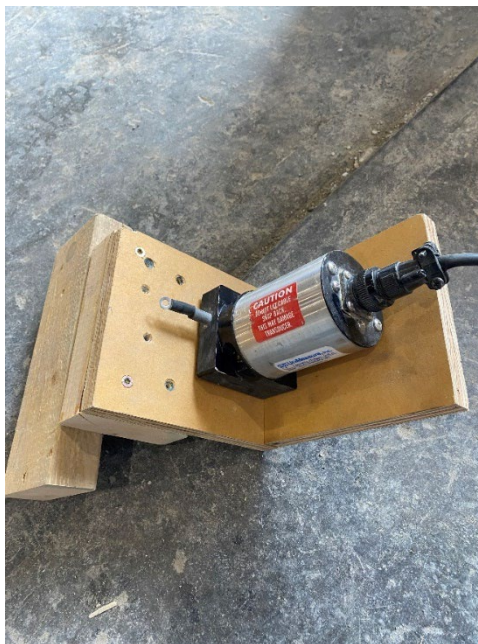
Figure 4.4 String potentiometer used to measure the transverse translation near the ground surface
