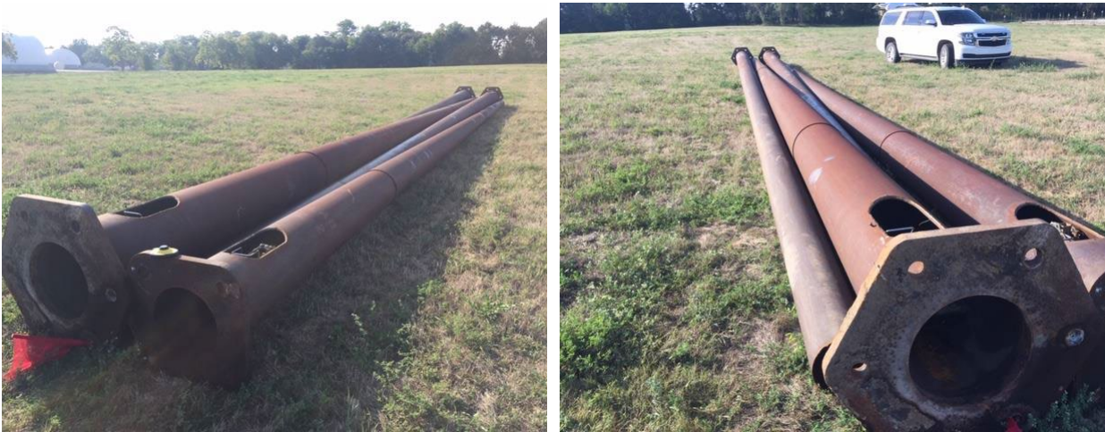
Figure 3.2 Tested poles in the field before installation
