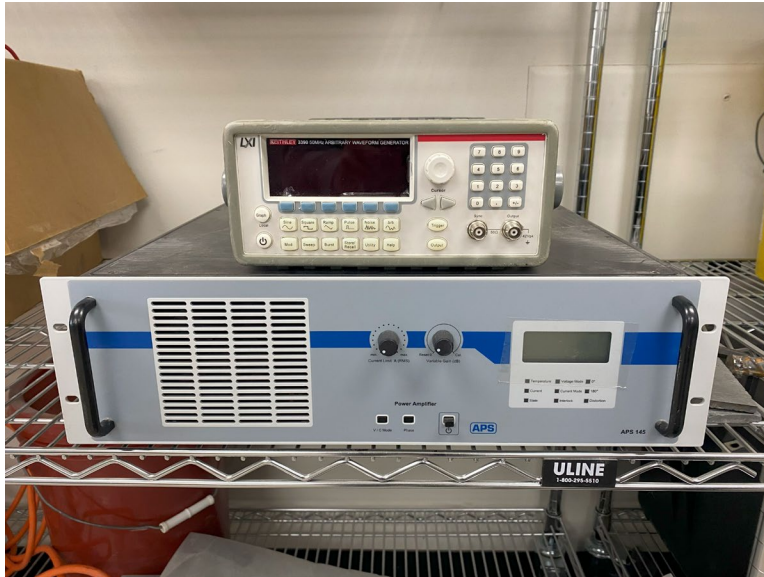
Figure 4.17 The APS 145 power amplifier and the signal generator used in the forced vibration test
