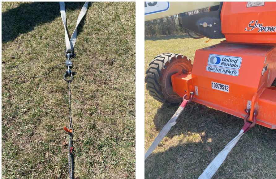
Figure 4.8 Pull setup for static and pluck tests
