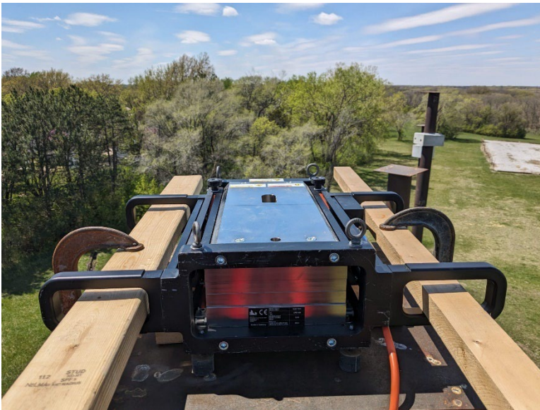
Figure 4.16 Installation of the shaker at the top of each pole before the forced vibration test
