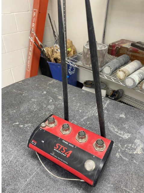
Figure 4.5 STS404 Wireless Intelliducer Node
