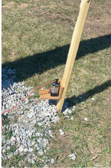
Figure 4.9 Measuring the transverse translation near the ground surface using a string potentiometer for static tests
