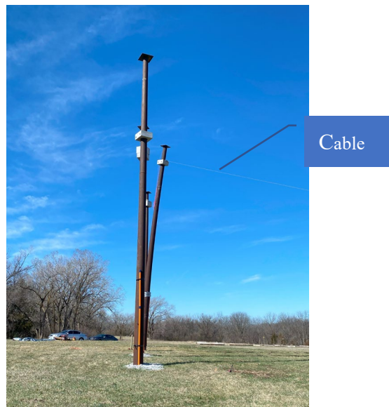
Figure 4.10 Static test (one direction)
