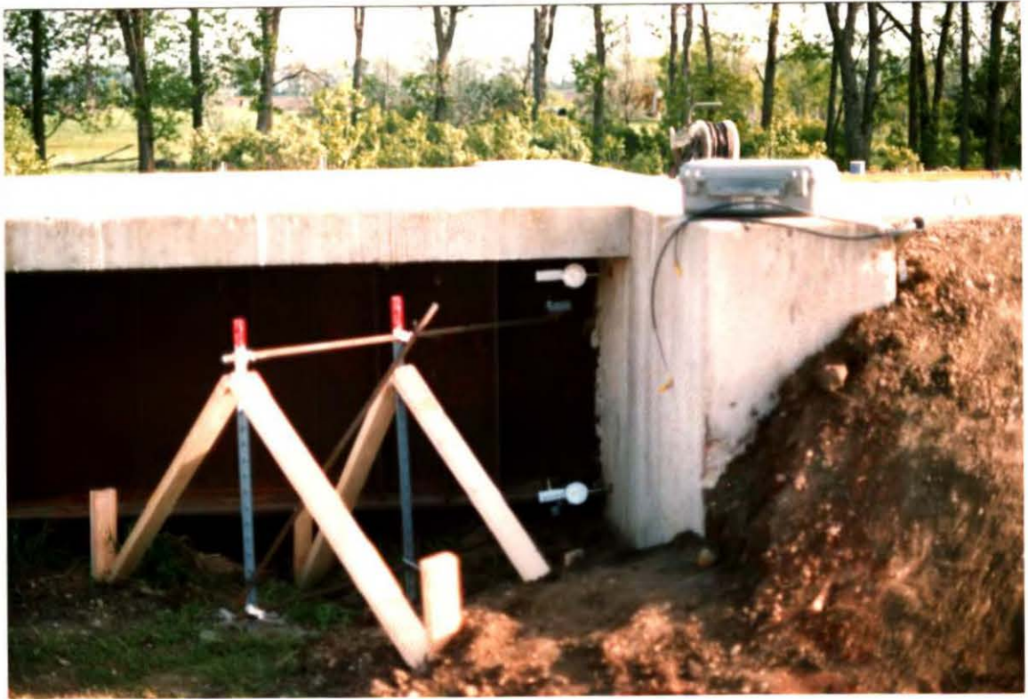
a. Dial gages positioned in front of abutment to measure movement and rotation of the abutment.
