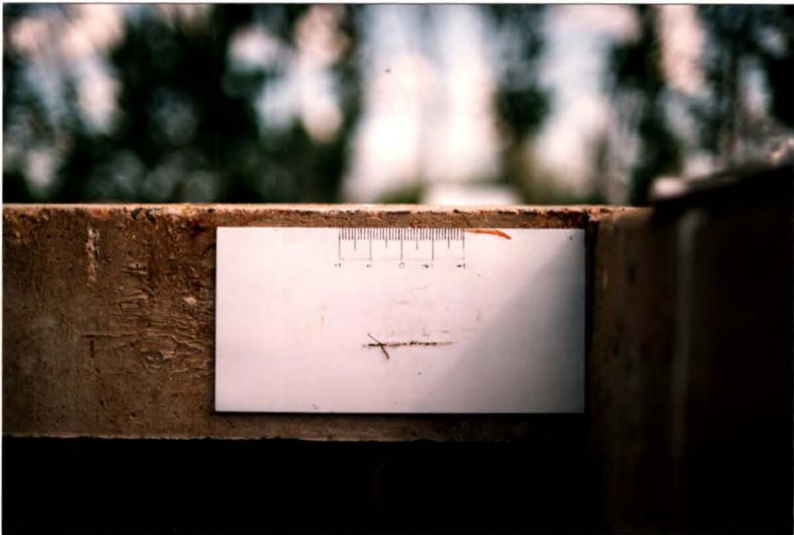
b. Plate used for monitoring abutment movement with a theodolite.
