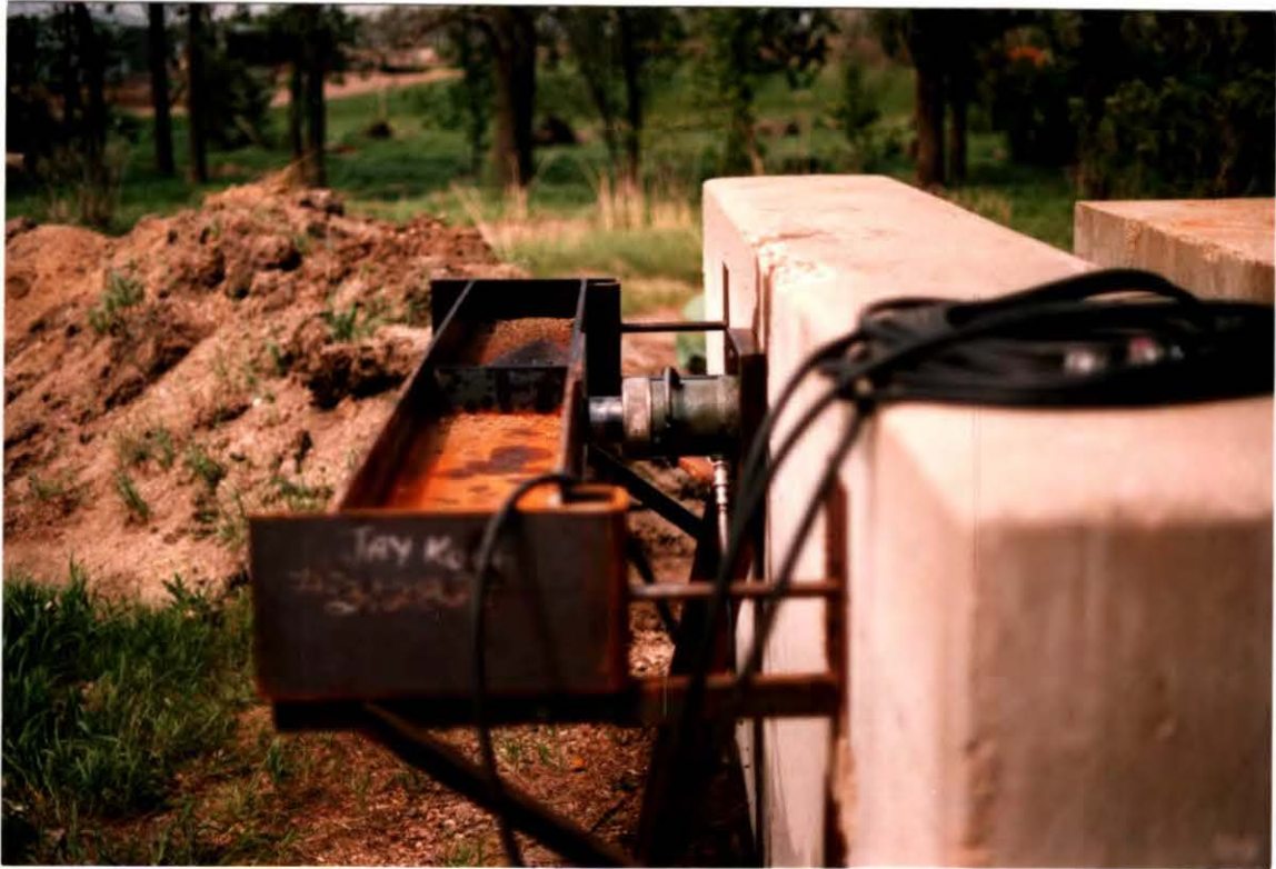
a. Jacking system at west end of reaction abutment to pull abutment wall away from the approach fill.
