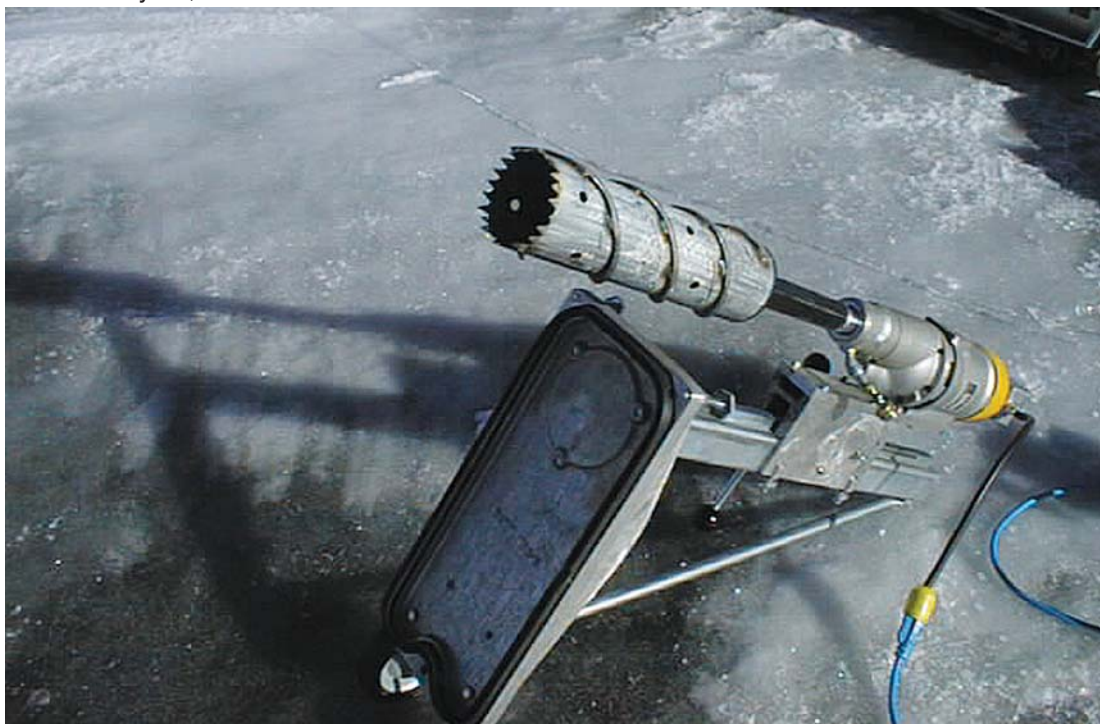
A Ice-coring machine with 4-inch coring bit attached at site 5 (Oahe Reservoirs near Mobridge) on February 12, 1999
