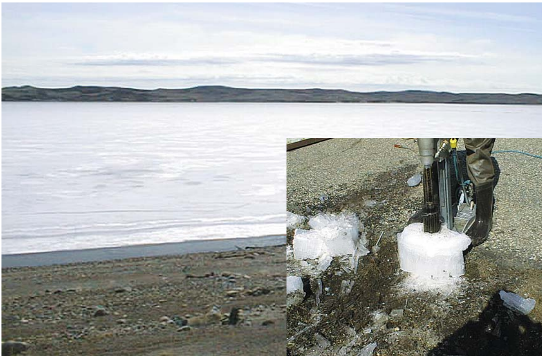
D Open water near shore at site 5 (Oahe Reservoir near Mobridge) on March 21, 2001. Ice chunks were collected by wading out to the ice mass. Samples were collected using the core drill on collected ice chunks.
