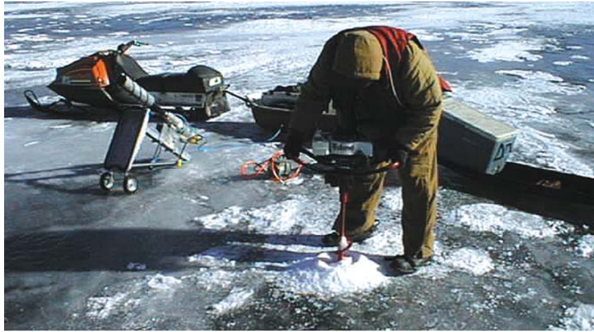
A Drilling hole for measuring ice thickness at site 5 (Oahe Reservoir near Mobridge) on February 12, 1999
