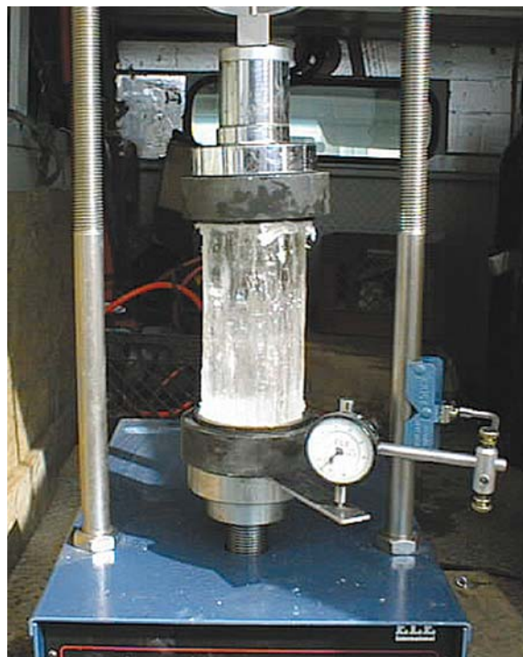
D Measurement of ice-crushing strength (note strain gage used to measure loading rate) at site 1 (James River at Huron) on April 2, 2001
