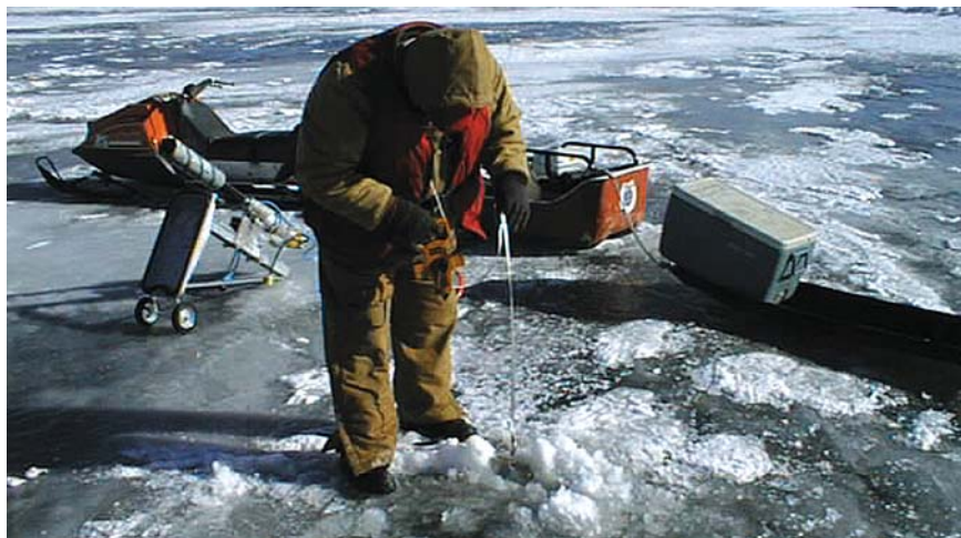
C Tape used to measure ice thickness (note hinged bar at end of tape)
