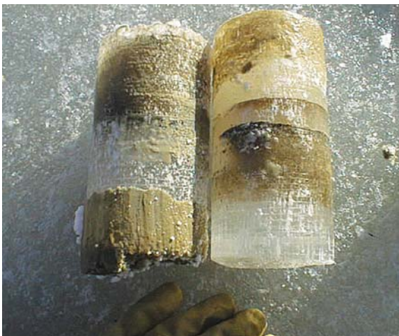
Figure 15. Photographs of samples collected for measuring ice-crushing strength at ice-data collection sites in South Dakota.
