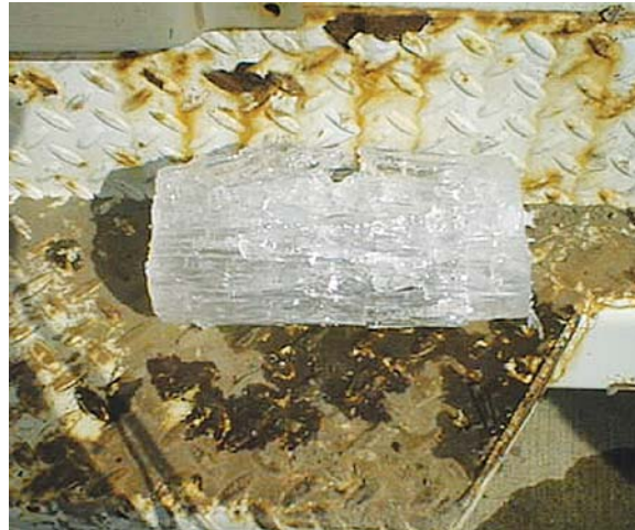
C Ice sample with alternating clear and sediment-mixed layers at site 3 (White River near Oacoma) on January 10, 2001
