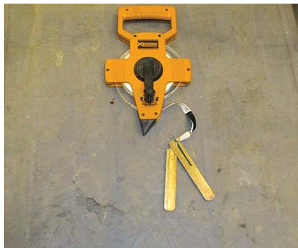
C Tape used to measure ice thickness (note hinged bar at end of tape)
